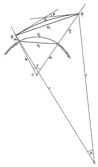
Figure 4: Reduction of wave path length  $d_1$  to ellipsoidal arc length  $d_4$  with the aid of the elevations ( $H_1$  and  $H_2$ ) of the terminals  $P_1$  and  $P_2$ . The wave path chord and the ellipsoidal chord lengths are denoted by  $d_2$  and  $d_3$ , respectively. The angle  $\gamma$  is subtended by the ellipsoid normal of radius R and through the terminals of the line. Similarly, the angle  $\beta$  is subtended by the normal to the wave path with radius r (Rüeger, 1996).
