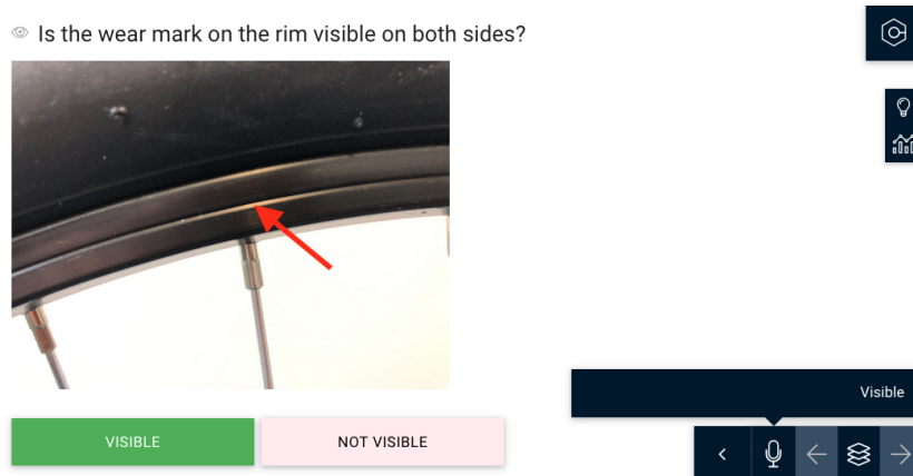
Fig. 4. The diagnosis interface of the Service Mate showing a specific question, a helpful image and the possible answers for the question as touch buttons. It is also possible to answer the question by speech input.
